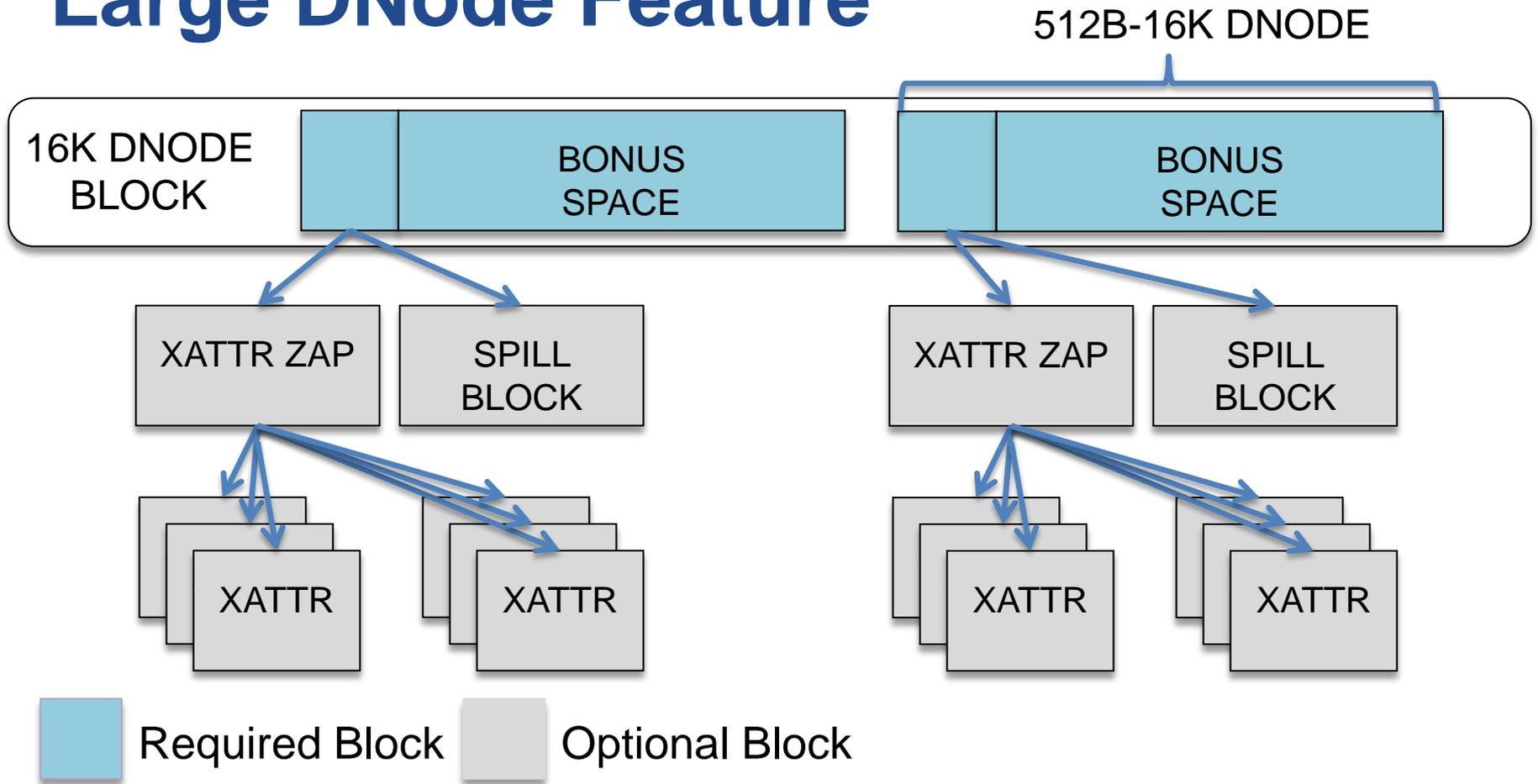
Only a single I/O is needed to read multiple dnodes with xattrs
