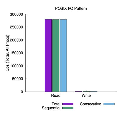
sequential: An I/O op issued at an offset greater than where the previous I/O op ended.
