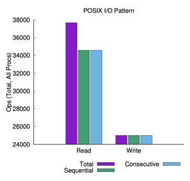
*sequential*: An I/O op issued at an offset greater than where the previous I/O op ended. *consecutive*: An I/O op issued at the offset immediately following the end of the previous I/O op.
