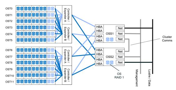
The diagram above represents a typical design for a high-availability object storage server cluster. It comprises two server machines, each with three network interfaces, and a storage array that is connected to each machine.
