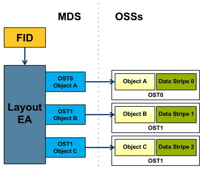
When a client wants to read from or write to a file, it first fetches the list of object FIDs containing the file's data from the MDT inode for the file. The client then uses this information to connect directly to the object storage servers where the data objects are stored and transact I/O on the file.
