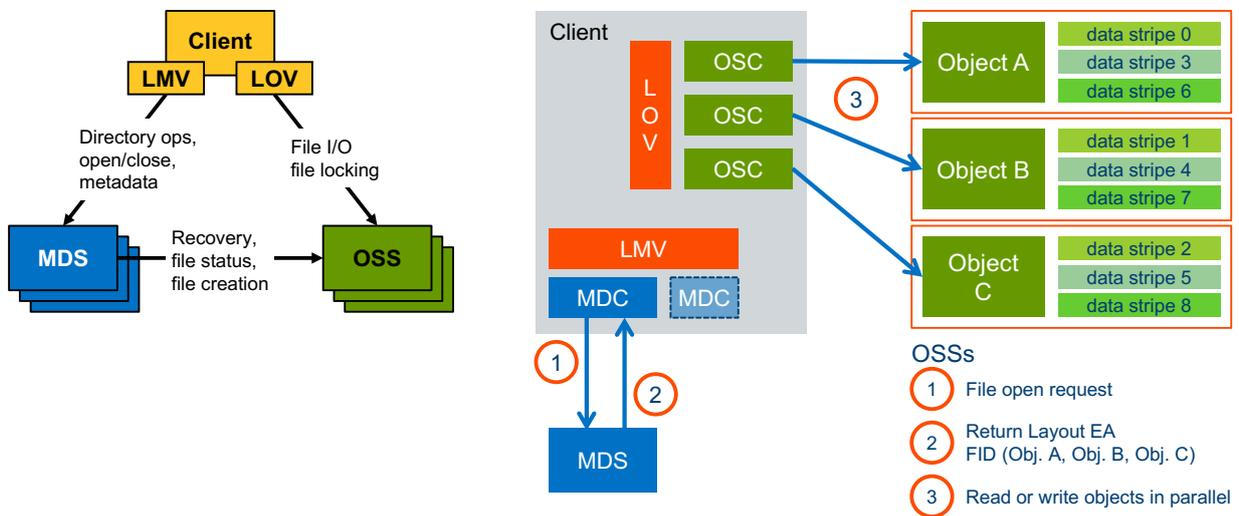
The Lustre client software provides an interface between the Linux virtual file system and the Lustre servers. The client software is composed of several different services, each one corresponding to the type of Lustre service it interfaces to. A Lustre client instance will include a management client (MGC, not pictured), one or more metadata clients (MDC), and multiple object storage clients (OSCs), one corresponding to each OST in the file system.
