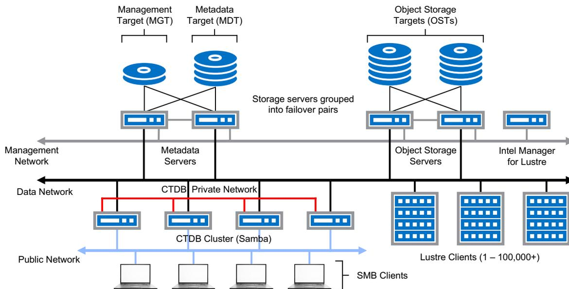
Lustre was originally designed for HPC applications running on large clusters of Linux-based servers and can present extremely high-capacity file systems with high performance. As it has matured, Lustre has found roles in IT system infrastructure, and has become increasingly relevant to commercial enterprises as they diversify their workloads and invest in massively-parallel software applications.
